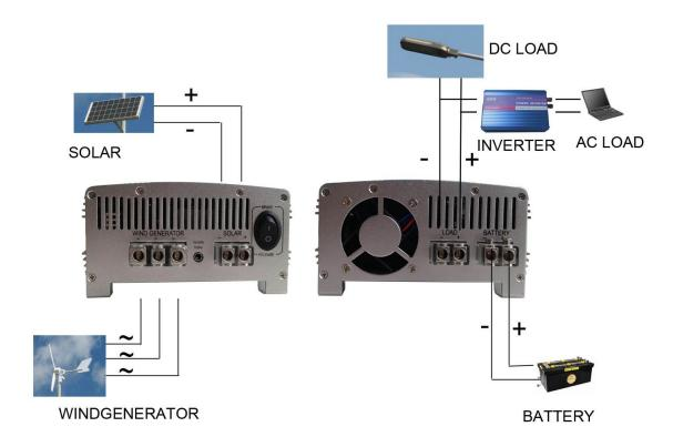
The distance between wind turbine and the charge controller, charge controller and battery should be as short as possible.
