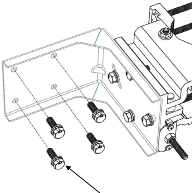
Attach 4 – 15mm M8 Bolts with flat and split lock washers to your MetroLinq unit
