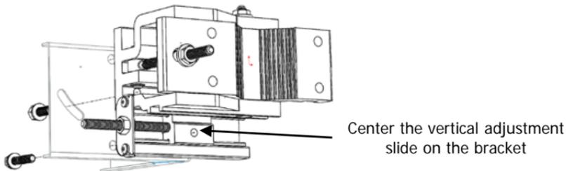
Attach 3 – 25mm M8 Bolts with flat and split lock washers to between the L-Bracket and Adjustment Assembly
