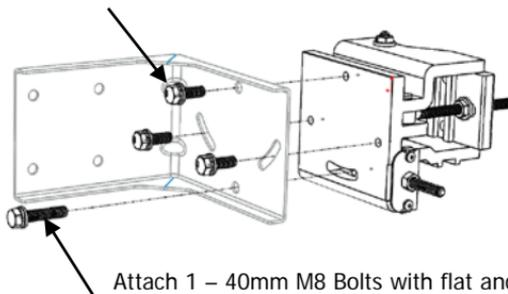
Attach 1 – 40mm M8 Bolts with flat and split lock washers to between the L-Bracket and Adjustment Assembly
